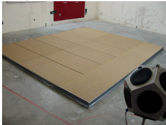
Wallpanel, thickness 40 mm, under test
