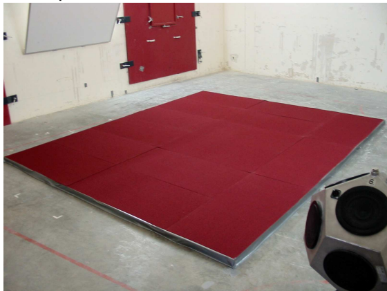
Wallpanel, thickness 20 mm, under test
